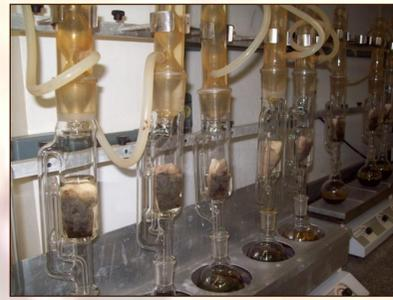
Figura 3: Extrator Soxhlet.
