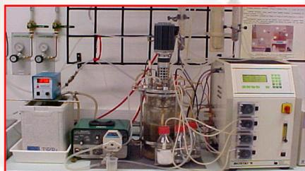
Figura 3. Biorreator de mistura completa (Biostat B®).
