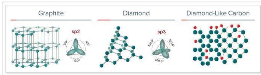
Fig 1. Structural difference between graphite, diamond and DLC[1]
